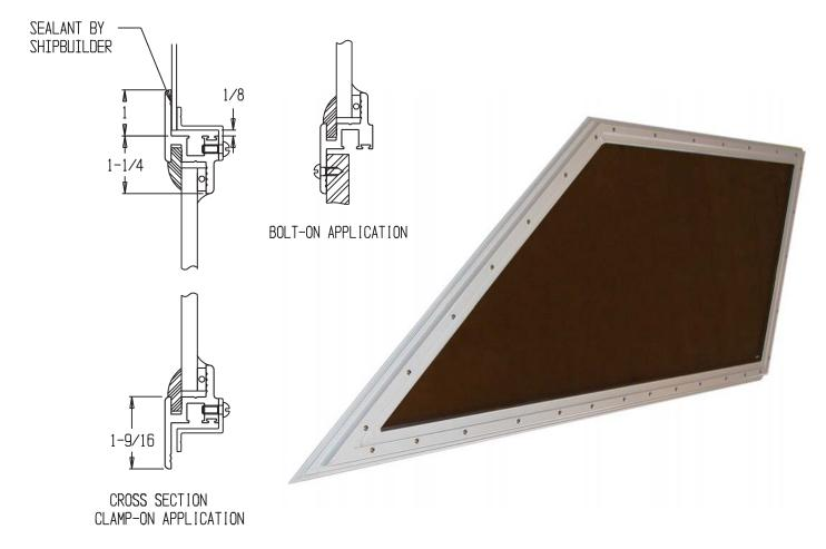
This fixed aluminum medium frame window has a clamp or bolt-on style frame and available in custom shapes and sizes. It will suit a glass thickness of 6 to 12mm. Heated glass is optional. Standard 3" radius corners [4" and mitered are optional] ABS type approved.
