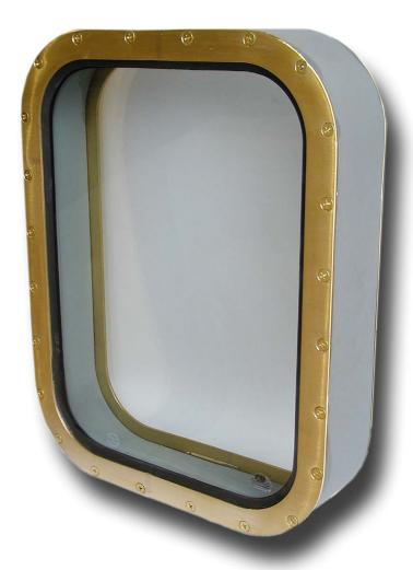
This heavy marine all weld-in mild steel or stainless steel fixed watertight window is available in custom shapes and sizes. The steel window frame is usually sandblasted and weld-able primer to suit most specifications. The stainless is either 304 or 316 grade.
